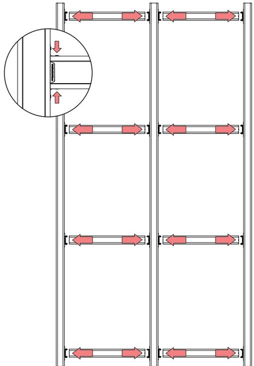
Creating and decorating aluminium framework has never been faster or more flexible. With only one profile required and adaptable connectors, the Stratlock Rail System is a foolproof way to create a consistent substrate for the perfect panel finish. For further information or technical support contact: [info@fastmount.com](mailto:info@fastmount.com)
